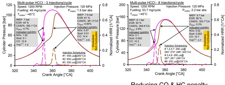
Relatively high CO & HC penalty due to large injection quantity/shot; Use of heavy EGR to improve combustion phasing Reducing CO & HC penalty with 8 Injections/ cycle; Higher boost and heavy EGR to improve LTC
