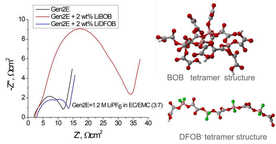
Density functional calculations show that fluorine termination prevents 3-D polymeric structure growth. This explains the low observed impedance for LiDFOB compared LIBOB
