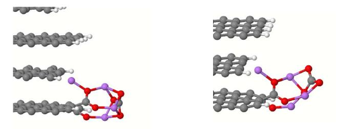
Defect sites (missing hydrogens) on the graphite edges are very reactive towards Li<sub>2</sub>CO<sub>3</sub> and are likely nucleation sites for lithium carbonate SEI growth.
