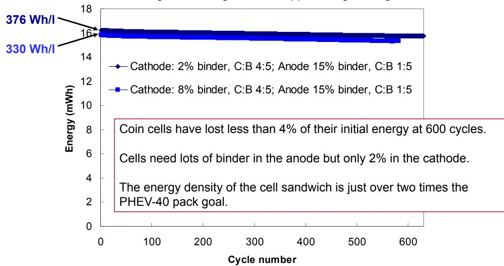
Energy density calculations include ½ of curr. coll., electrodes, and separator.
