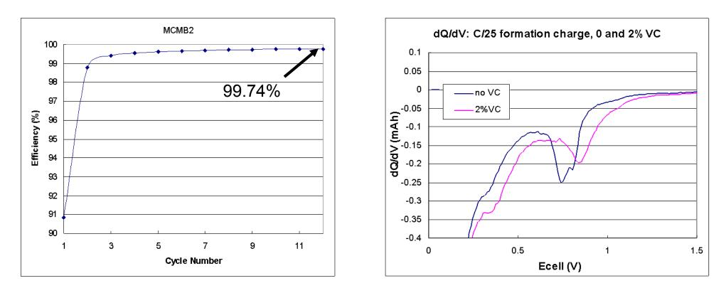
To get to 2500 cycles with just 20% capacity loss, we need coulombic efficiencies of
