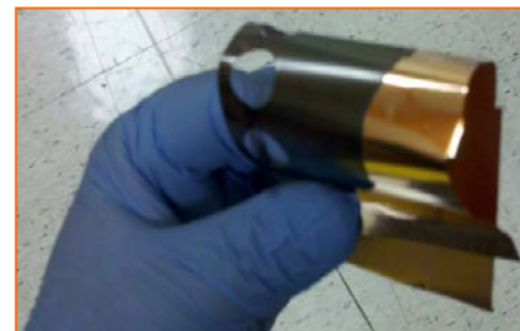
Flexible anode with good adhesion
