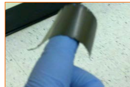
Flexible free standing \sim 65 \mu\text{m} anode composite after calendering
