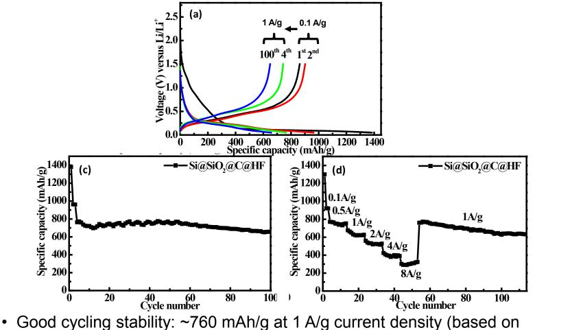
the total electrode weight, including binder and conductive carbon)
