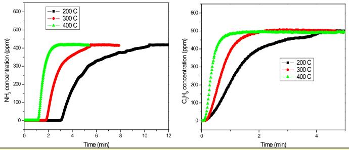
• SCR catalyst shows significant adsorption capacity for NH<sub>3</sub>, C<sub>3</sub>H<sub>6</sub>, C<sub>2</sub>H<sub>4</sub> and CO
