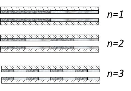
Arrangement of LNT(Pt/BaO/Al<sub>2</sub>O<sub>3</sub>) and SCR(CuZSM5) catalysts; n is the number of combined LNT+SCR units. Catalysts are divided equally in each arrangement .
