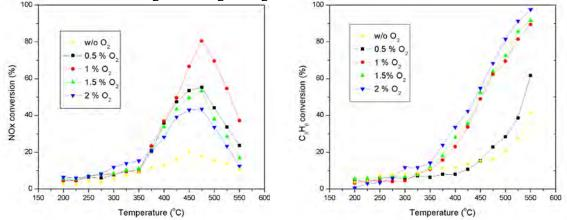
Cycle-averaged NOx reduction: 300 ppm NO, 8%  $O_2$  / 60 s L; 3333 ppm  $C_3H_6$ , 0 or 1%
