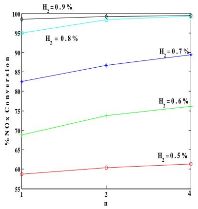
Conditions: Total length = 4cm; T =  $275^{\circ}$ C ; GHSV=60,000hr<sup>-1</sup>; Lean cycle (60 sec): 500ppm NO, 5% O<sub>2</sub>;
