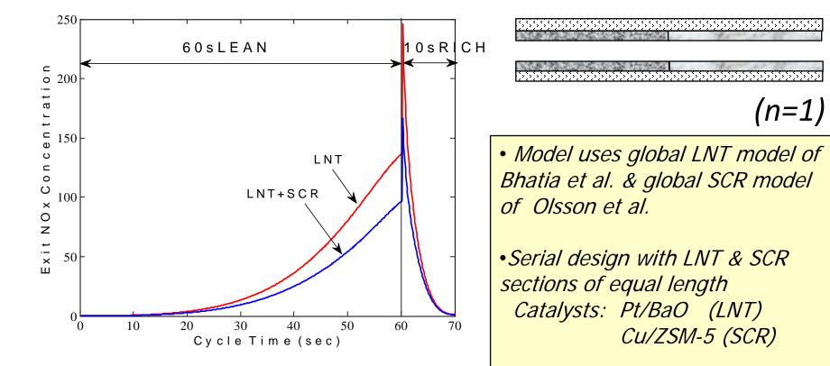
Length of each catalyst = 2cm; Temperature= $275 \circ C$ ; GHSV= $60,000h^{-1}$ ; Lean inlet: NO= $500ppm,O_2=5\%$ ; Rich inlet: NO= $500ppm,H_2=0.8\%$ ;
