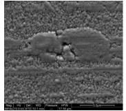
Some Metal transfer Tribofilm patches No surface damage
