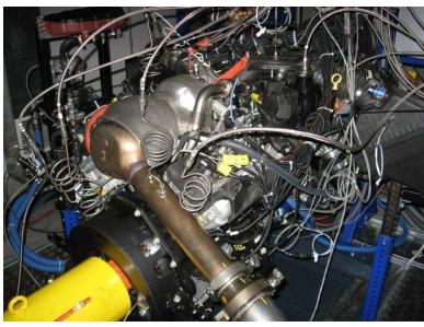
Base 4.5L V8 Diesel Engine Testbed
