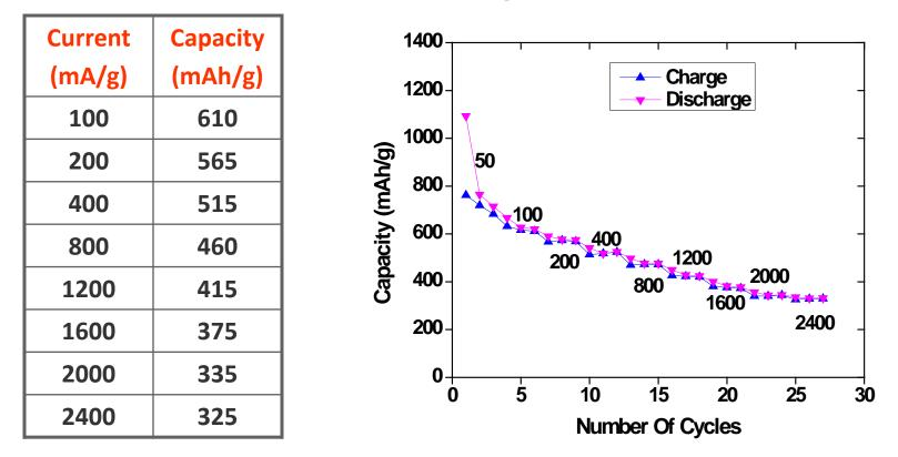
Good cycling with high coulombic efficiency after the first cycle.
