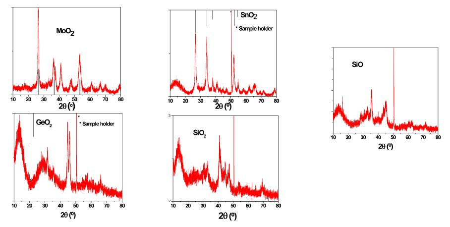
XRD shows that the SnO<sub>2</sub> structure was conserved, MoO<sub>3</sub> was reduced to MoO<sub>2</sub> and no trace of GeO<sub>2</sub> is present confirming the composite structure.
