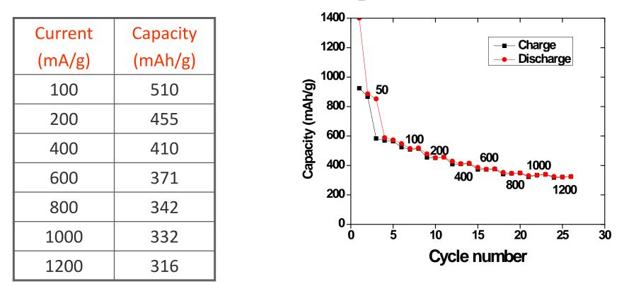
Good cycling with high coulombic efficiency (1<sup>st</sup> cycle irreversibility is about 65% due to the formation of Li<sub>2</sub>O which is not active in the case of SnO<sub>2</sub>-Sn<sub>30</sub>Co<sub>30</sub>C<sub>40</sub> composite).
