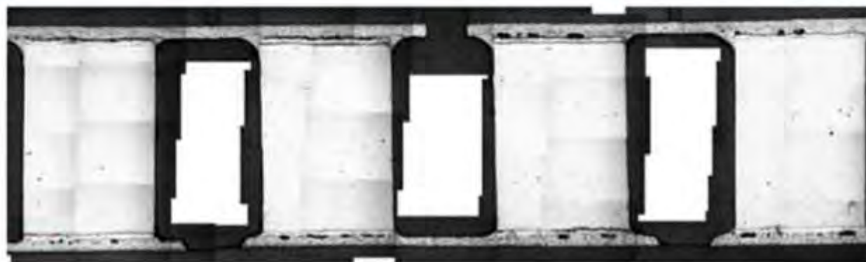
P&N Skutterudite on DBA ceramic (Thermal Cycled ~450C, 30x's)
