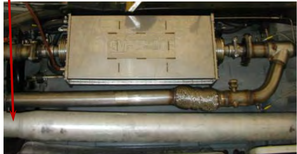
Front Center thermocouple on heat exchanger
