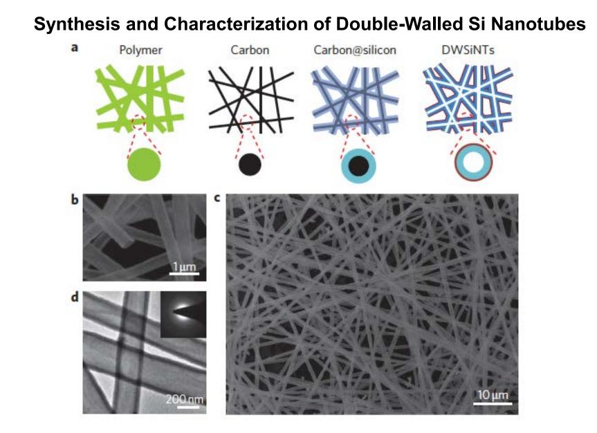
Characterization of Double-Walled Si Nanotubes by ex-situ transmission electron microscopy
