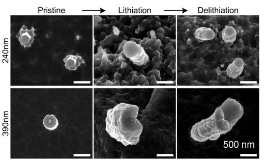
Large Si nanopillar is easy to break. Transition size: 240 ~ 360 nm Fast reaction enhances fracture
