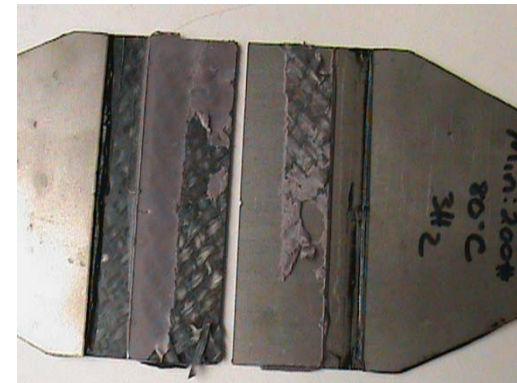
Fatigue failure “adhesive bond only” (80°C)
