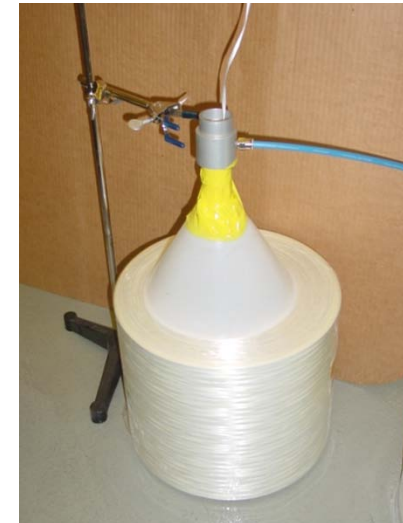
High Output Robotic Deposition Requires Significant Tow Spacing and Air Tensioning in Addition to Guides Implemented Previously
