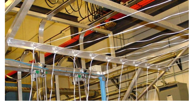
High Output Robotic Deposition Requires Significant Tow Spacing and Air Tensioning in Addition to Guides Implemented Previously
