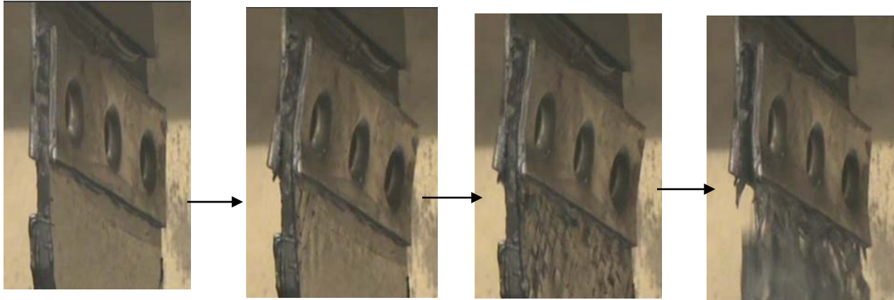
Damage progression during fatigue test of weld bonded specimen (video)
