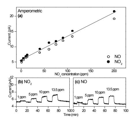
Test Temperature =  $600^{\circ}C$ Filter Temperature =  $400^{\circ}C$  $O_2$  level 3% in gas
