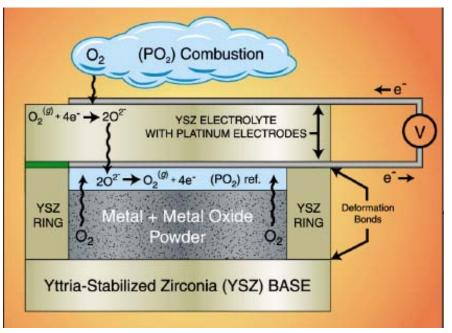
•At T>450° C, a specific oxygen partial pressure  $(pO_2)^{int.}$  from M+MO is generated within the sensor package.
