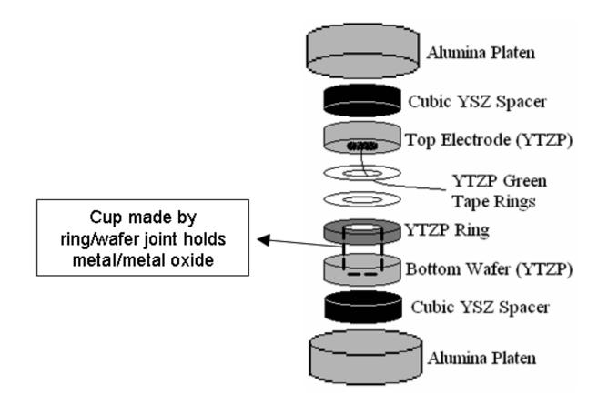
Sensor components are stacked and joined in a one-step process
