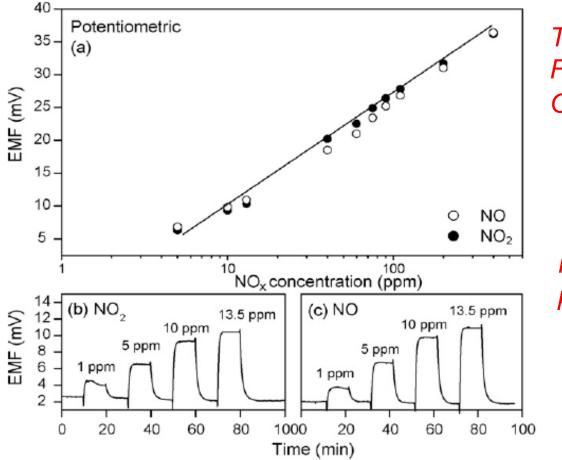
Test Temperature =  $600^{\circ}C$ Filter Temperature =  $400^{\circ}C$  $O_2$  level 3% in gas
