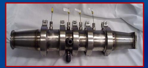
Modular testing allows to characterize the individual components in TWC
