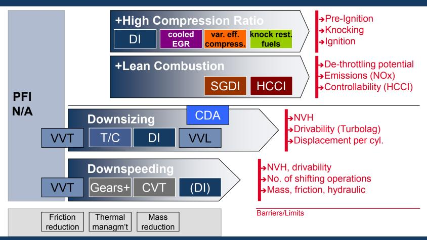
Due to new test cycles and trends towards downsizing and downspeeding, high compression ratios become more important to reduce CO2.
