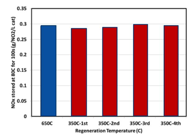
Cumulative NOx stored on the CSC<sup>™</sup> for the first 100 seconds at 80°C after regeneration at 650°C (blue bar) and subsequently after each repeated regenerations at 350°C (red bars)
