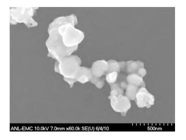
Phase pure copper nanoparticles synthesized using an in situ chemical process (*D. Singh, et al., unpublished data*).
