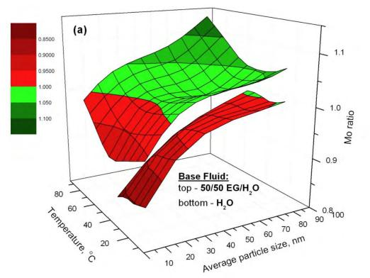
Effectiveness of heat transfer for 4 vol.% SiC in  $EG/H_2O$  and  $H_2O$
