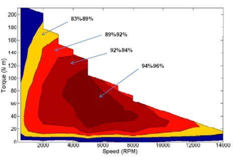
Figure 1. Motor Efficiency Targets
