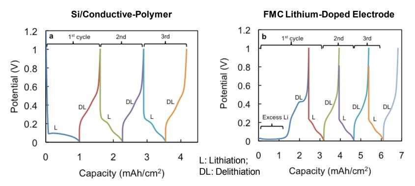
Excessive amount of FMC Lithium was used in our initial testing process. Upon assembling the cell, the Si electrode is fully lithiated. The FMC lithium-dope electrode begins from delithiation rather than lithiation in a normal Si electrode.
