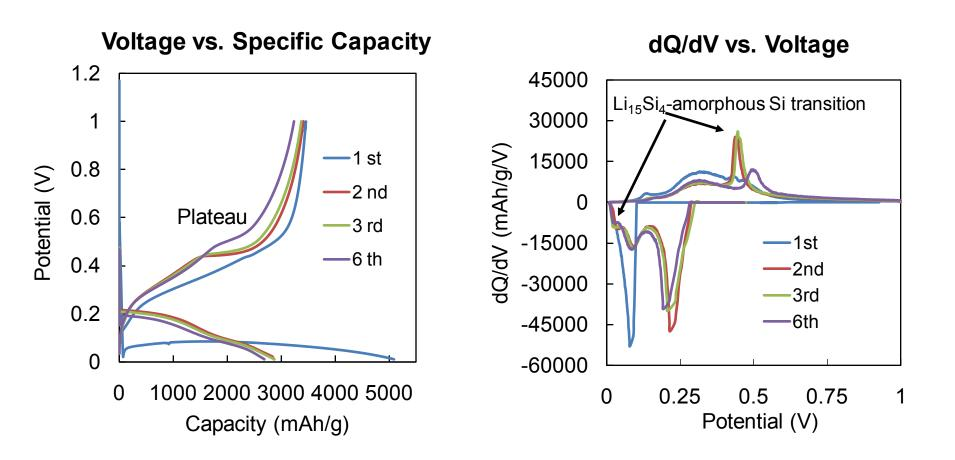
Si Nanoparticles experience same phase transition as micron size particles.
