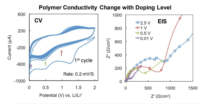
The electronic conductivity of the binder increases during Li-ion doping .
