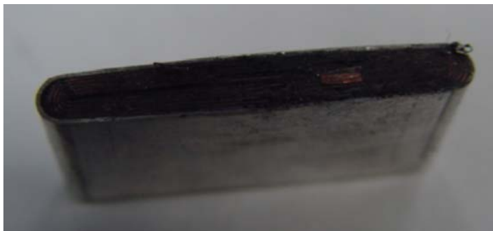
A cross-section of a discharged cell showing the aluminum casing and the “jelly roll”.
