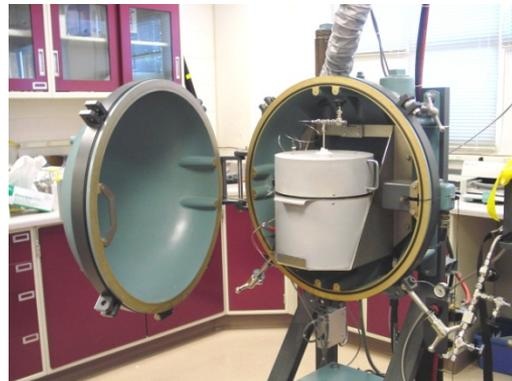
Accelerating Rate Calorimetry
