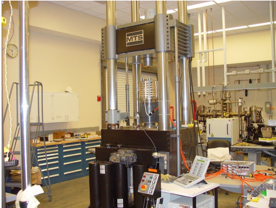
Four-post MTS 500,000-lb. load frame shown with extrusion tooling
