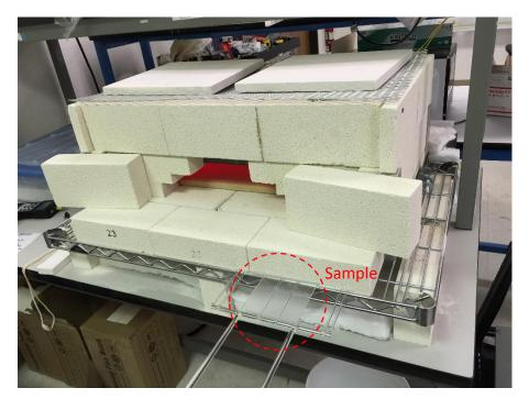
Figure 10 – Proof of Principle IR Cure Oven
