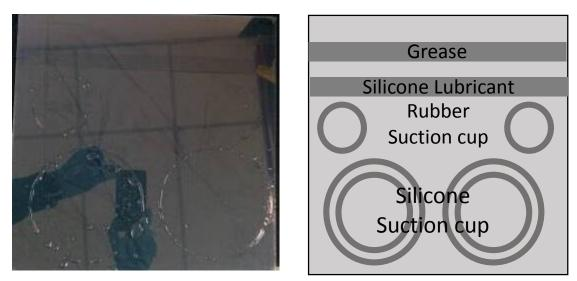
Fig 1. Surface Treatment Sample Preparation
