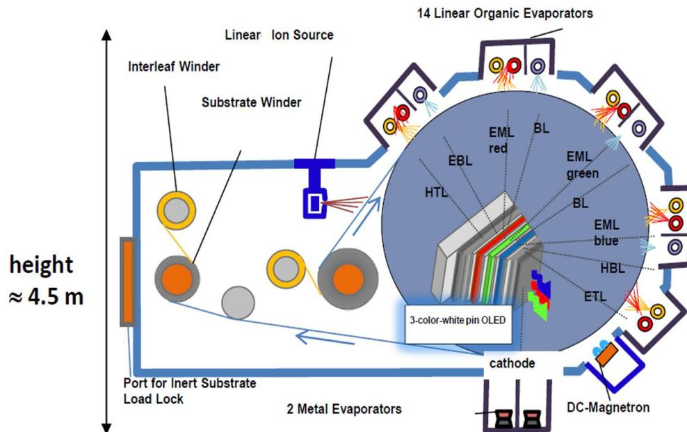
**Figure 6.16 R2R OLED Deposition Line in Dresden**
