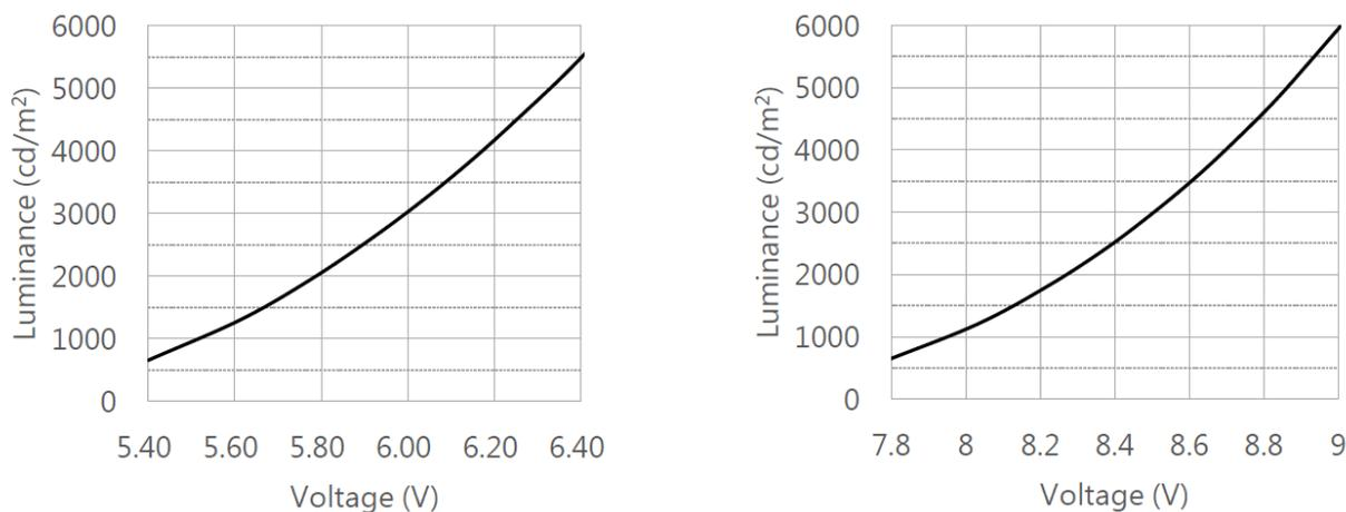
**Figure 6.2 Luminance vs Voltage for a 2-stage Panel (left) and 3-stage Panel (right) from LG Chem**
