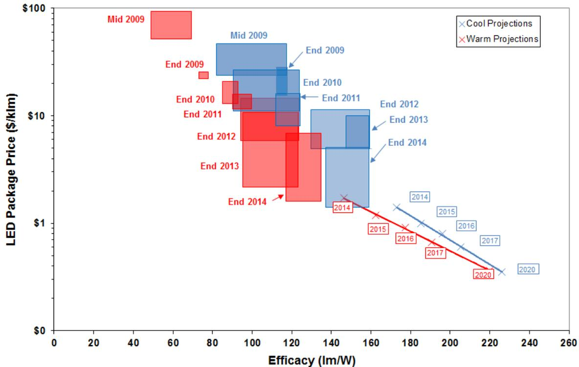
**Figure 5.17 Price-Efficacy Trade-off for LED Packages at 1 W/mm<sup>2</sup> (equiv. 35 A/cm<sup>2</sup>) and 25°C**
