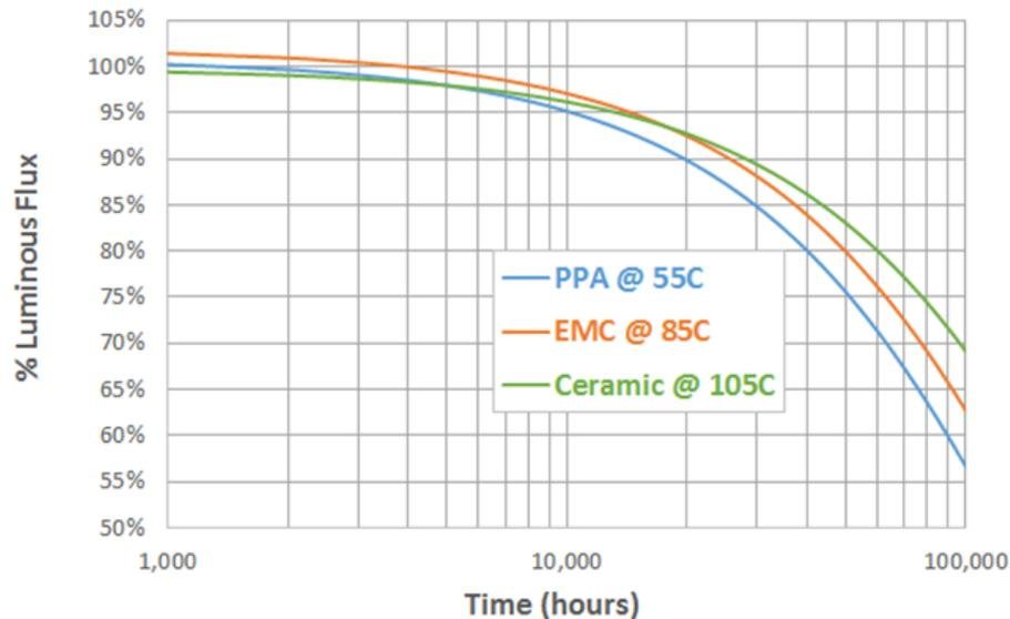
**Figure 5.14 Lumen Degradation Performance of Mid-Power Packages (PPA and EMC Plastic Resins) and High Power Packages (Ceramic Substrates).**
