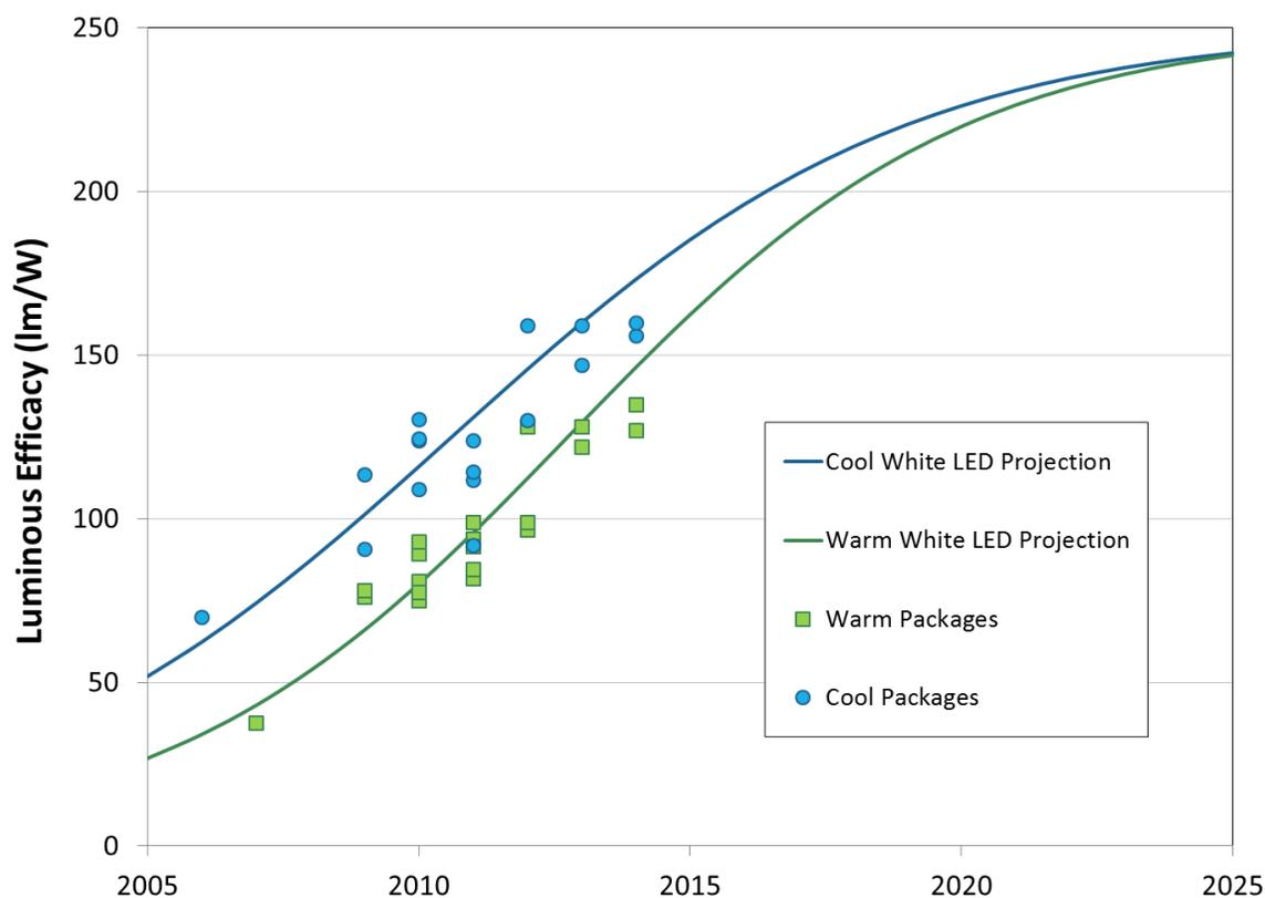
Figure 7.2 LED Package Efficacy Projections for Commercial Products
