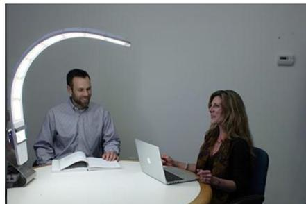
**Figure 2.4 Combination of Ambient, Surround and Task Lighting for Efficient Office Lighting**
