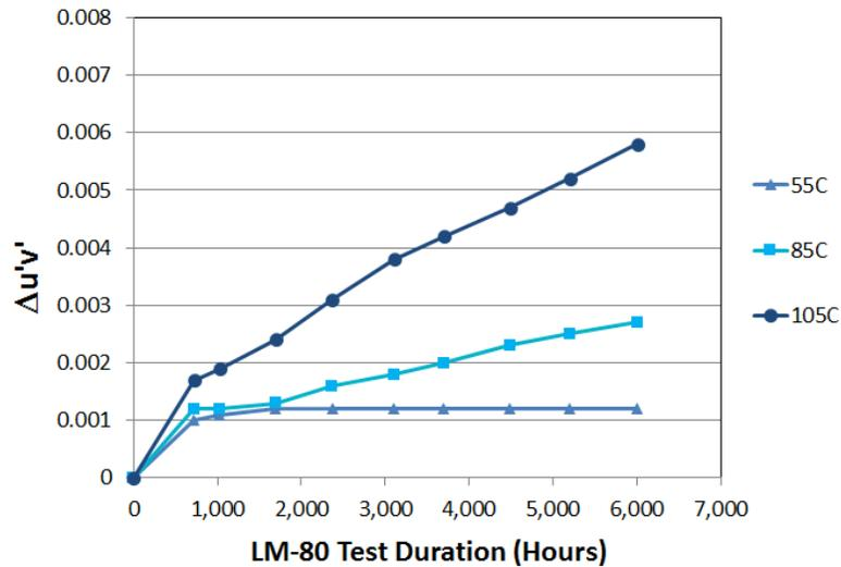
**Figure 5.15 Color Shift of LED Package as a Function of Temperature**
