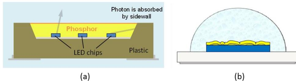
**Figure 5.13 LED Package Schematics Showing (a) Sidewall Discoloration and (b) Phosphor Delamination.**
