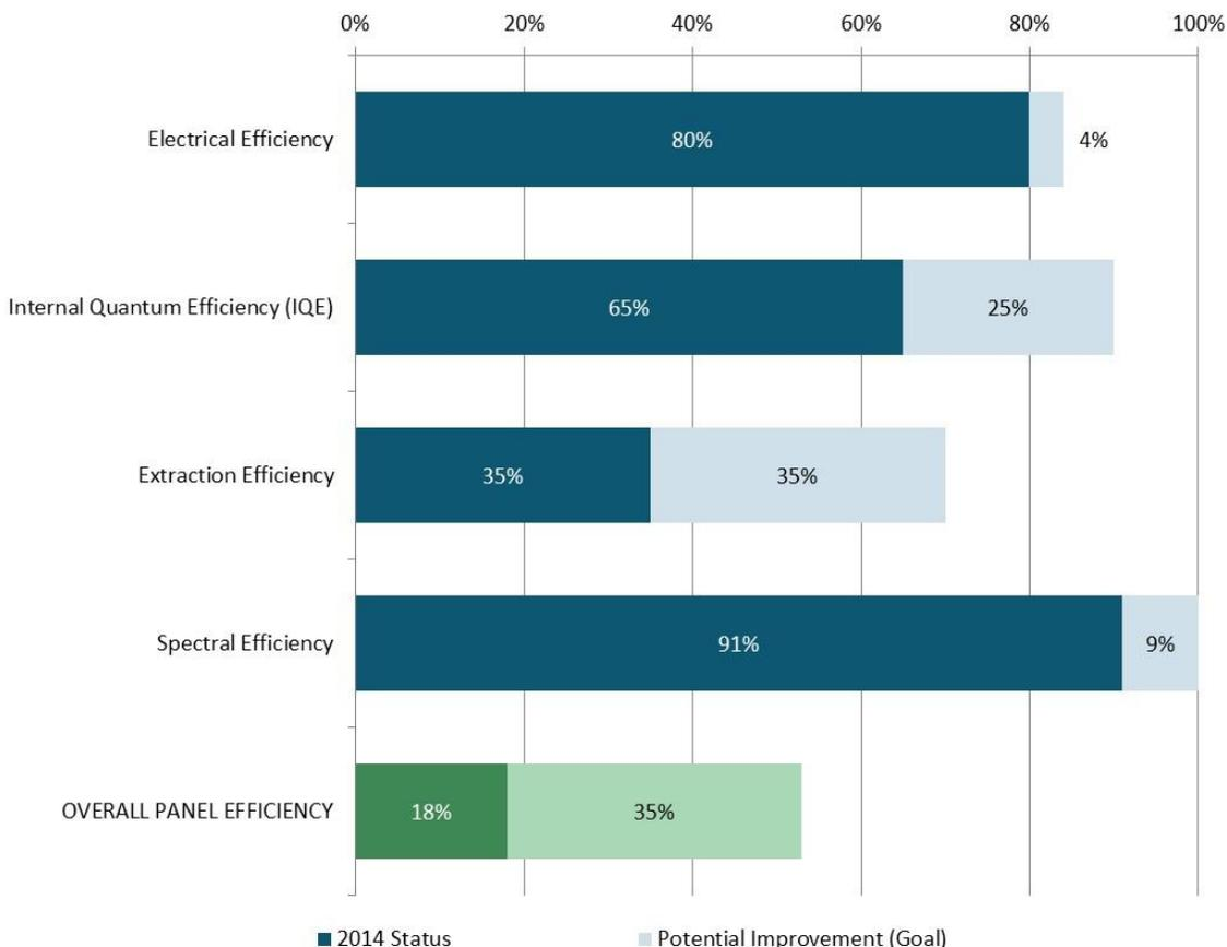
**Figure 6.4 OLED Panel Loss Channels and Efficiencies**
