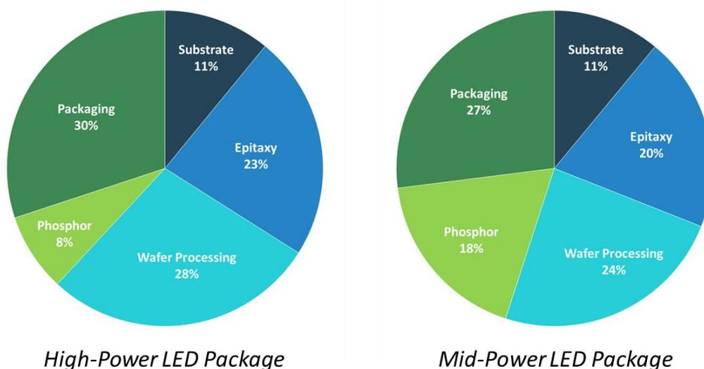
**Figure 5.9 Typical Cost Breakdowns for High-Power and Mid-Power LED Packages**
