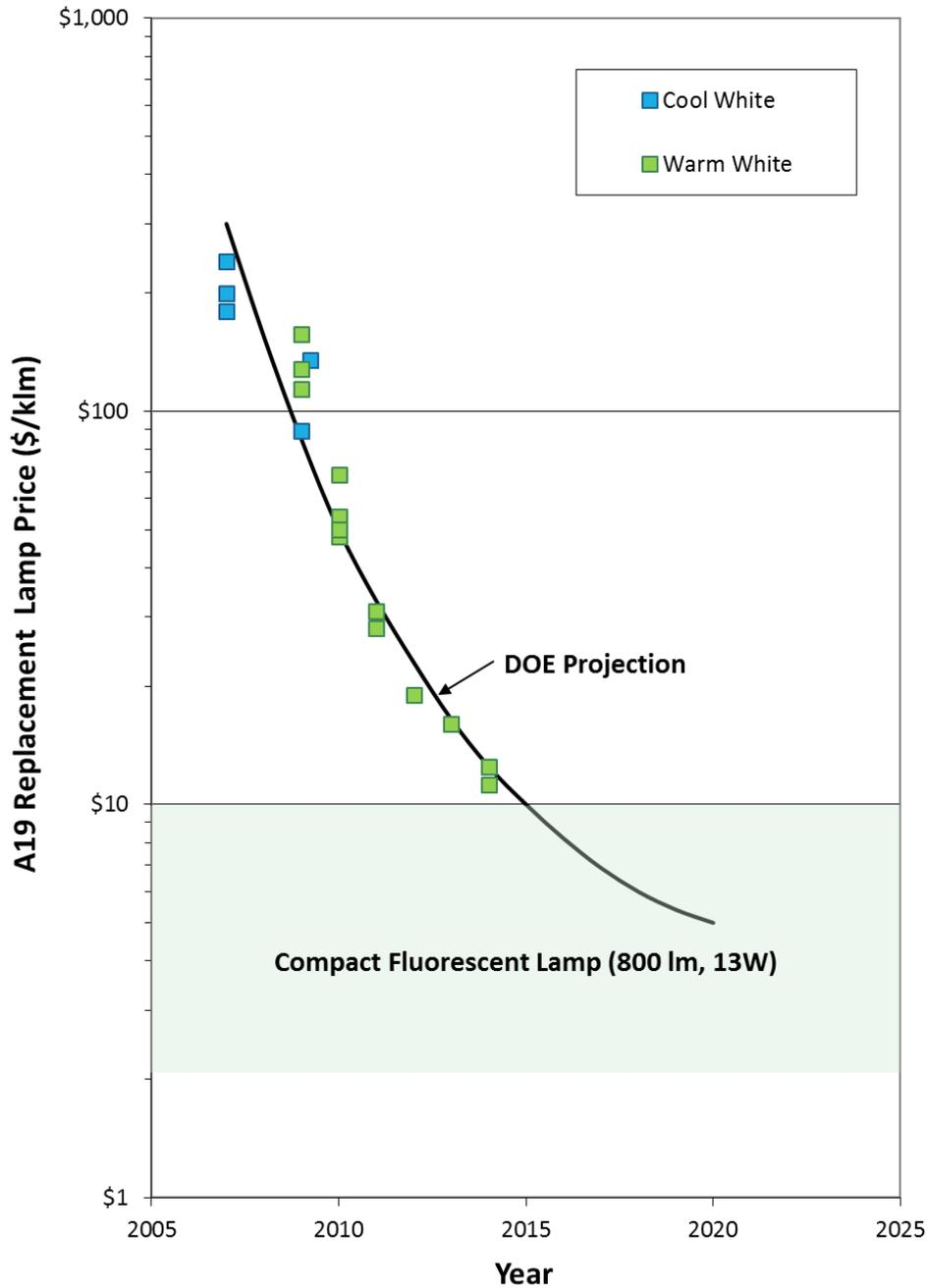
**Figure 5.18 A19 Replacement Lamp Price Projection (60W Equivalent; Dimmable)**
