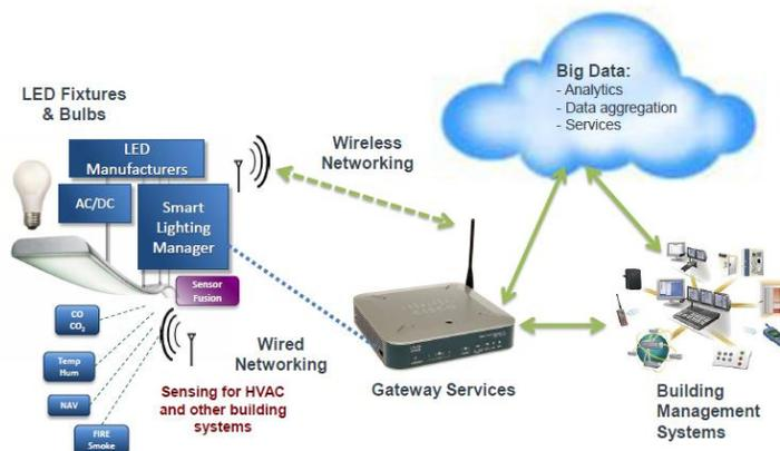
**Figure 2.7 Lighting as Part of an Integrated Control System**
