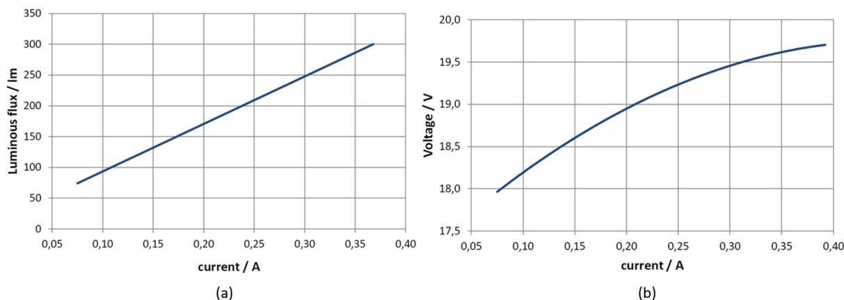
**Figure 6.3 Dependence of Luminous Flux and Drive Voltage on Current**
