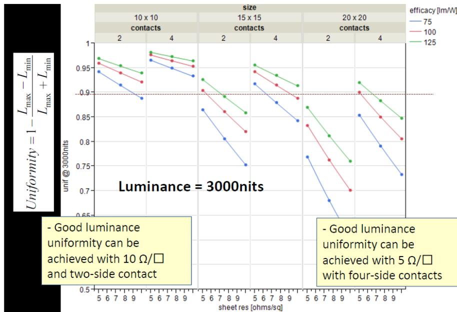
**Figure 6.18 Luminance Uniformity as a Function of Anode Sheet Resistance**
