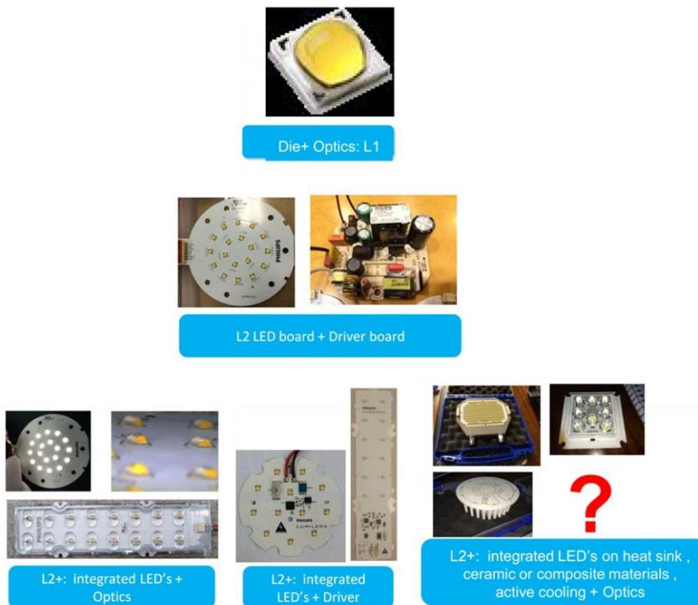
**Figure 5.6 Integration Path for LED Components**
