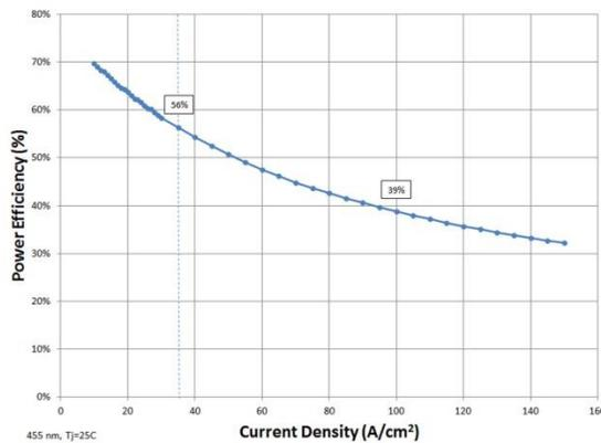
(b) Typical current efficiency droop (Cree XT-E)
