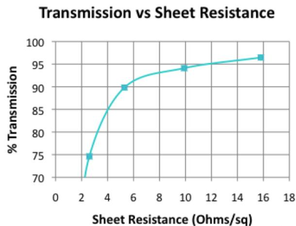
**Figure 6.19 Optical Transmission vs Sheet Resistance for Ag Nanowire Coatings**
