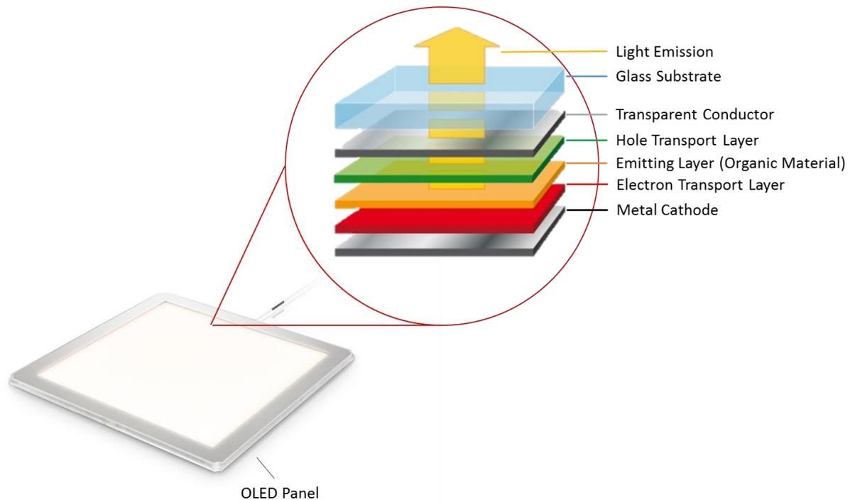
**Figure 8.2 Components of an OLED Panel**
