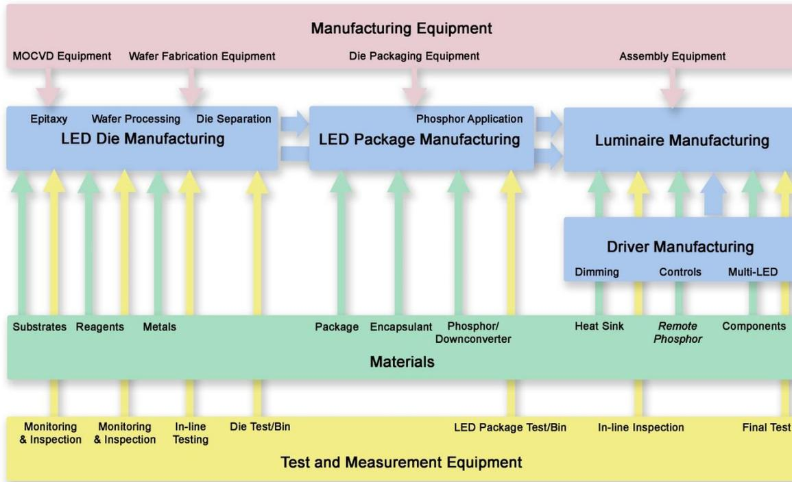
Note: The blue-shaded boxes and blue arrows describe the main manufacturing flow. The supporting elements of the supply chain are broken down into manufacturing equipment, materials, and test and measurement equipment. These supporting elements feed into the main manufacturing flow as indicated by the relevant arrows.
