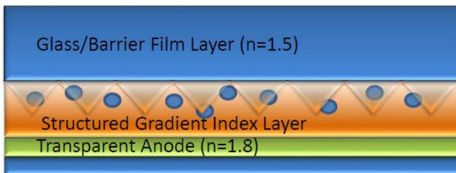
**Figure 6.20 Hybrid Light Extraction Layer with Graded Index**
