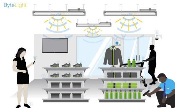
**Figure 2.11 VLC + BLE – Turn Lightings into Indoor Location Beacons**
