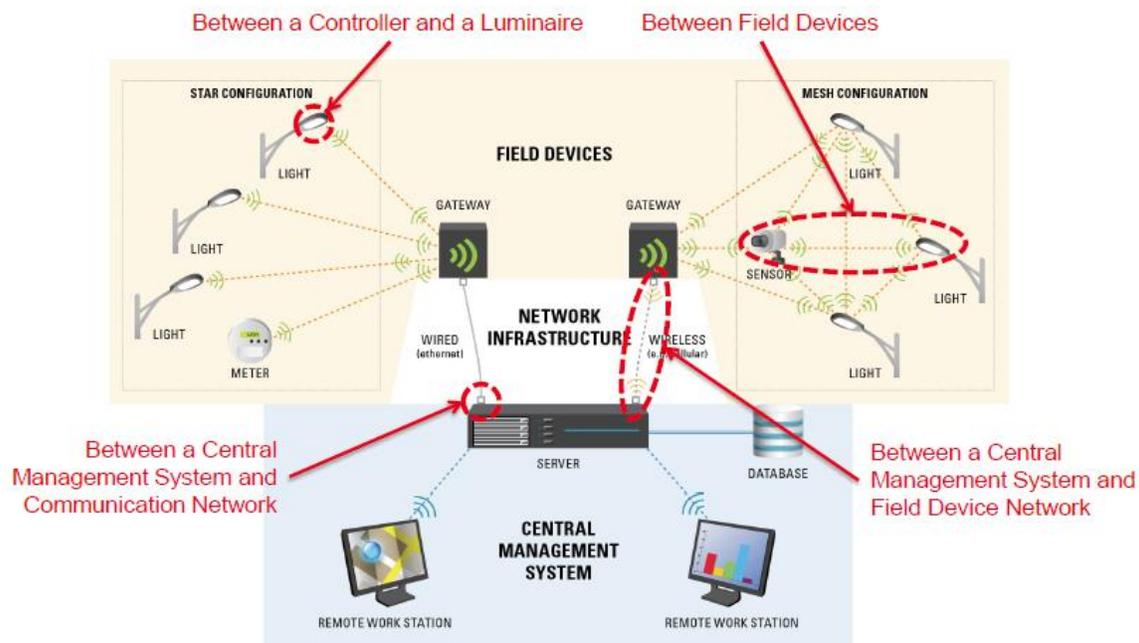
**Figure 2.8 Lights, Sensors, Meters, Gateways, and Management Systems Working Together**
