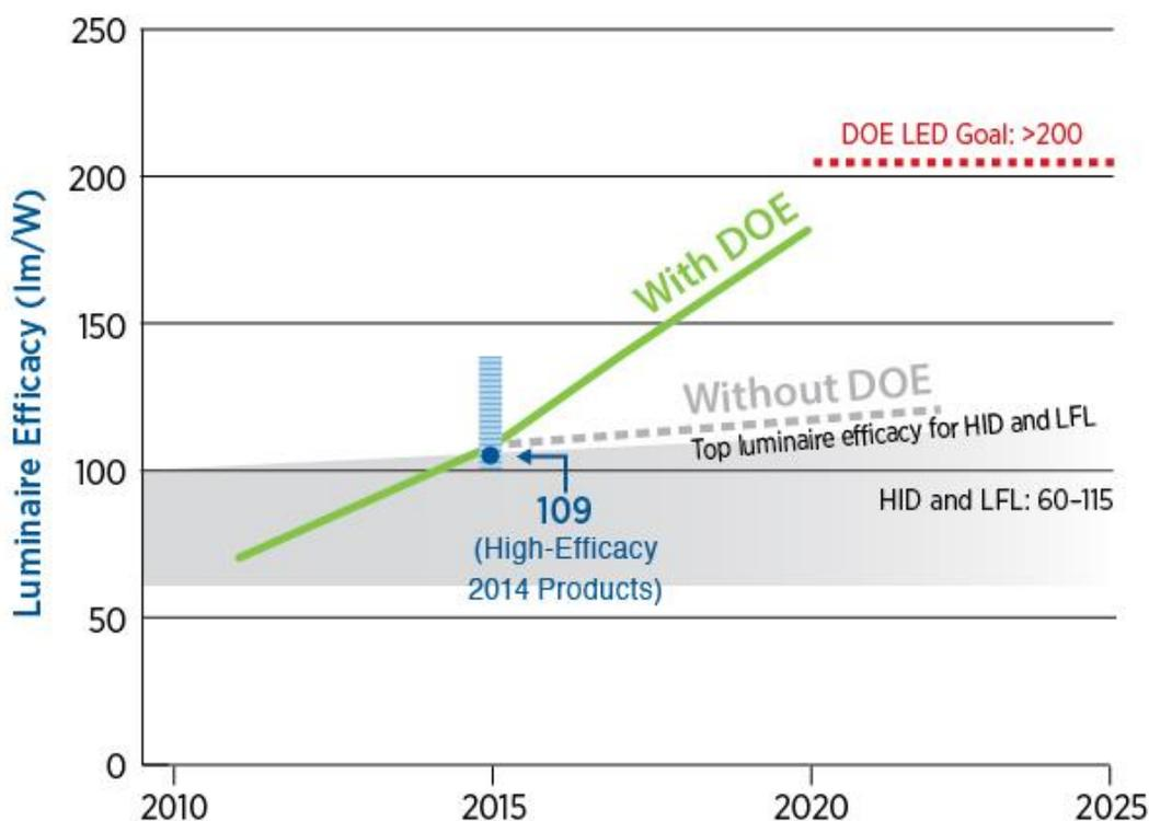
**Figure 2.1 Comparison of LED and Incumbent Light Source Efficacies**
