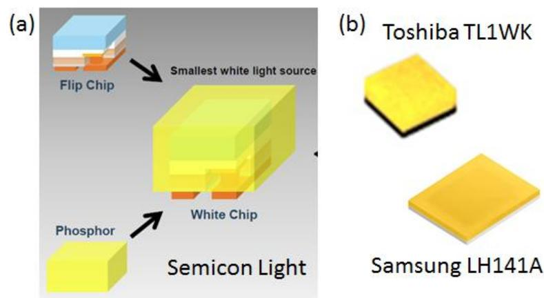
**Figure 5.8 (a) Schematic Representation of a CSP Manufacturing Approach and (b) Recent Examples of Commercial CSPs.**
