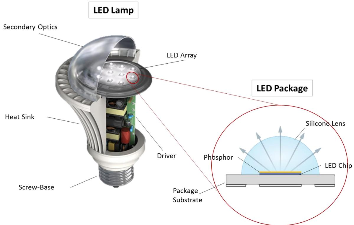
**Figure 8.1 Components of an LED Lamp**
