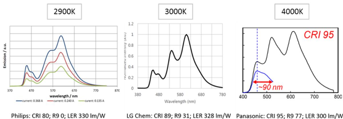
**Figure 6.1 Spectra of Commercial and Laboratory OLED Panels**
