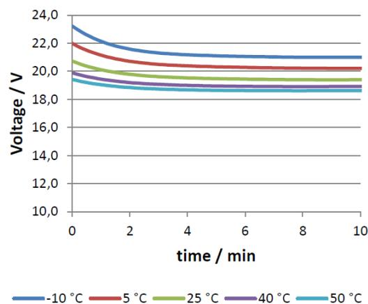
**Figure 6.22 Variation of OLED Drive Voltage with Ambient Temperature During Warm-Up Phase**
