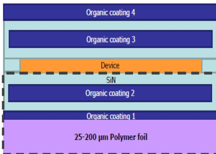
**Figure 6.21 Multi-layer Barrier Coating to Prevent Ingress of Moisture and Oxygen**
