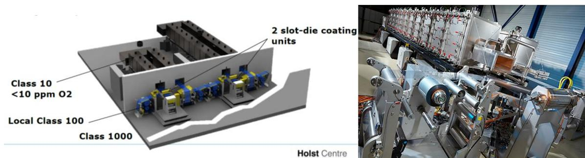
**Figure 6.17 R2R Pilot Line for Organic Electronics at the Holst Centre in Eindhoven**
