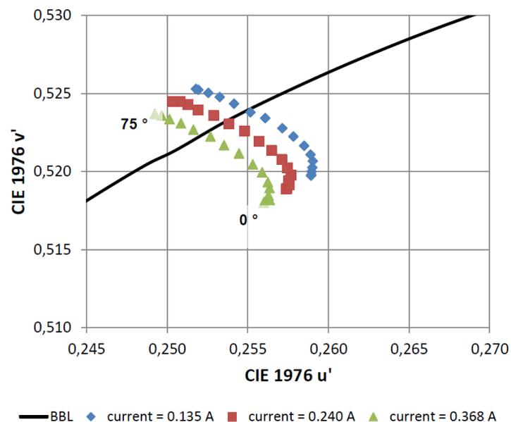
**Figure 6.5 Variation of Color Point on CIE1976 ( $u',v'$ ) Diagram with Drive Current and Emission Angle**
