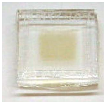
quartz/EVA/quartz specimen Kempe et. al., Proc. PVSC 2009, 1826-1831.
