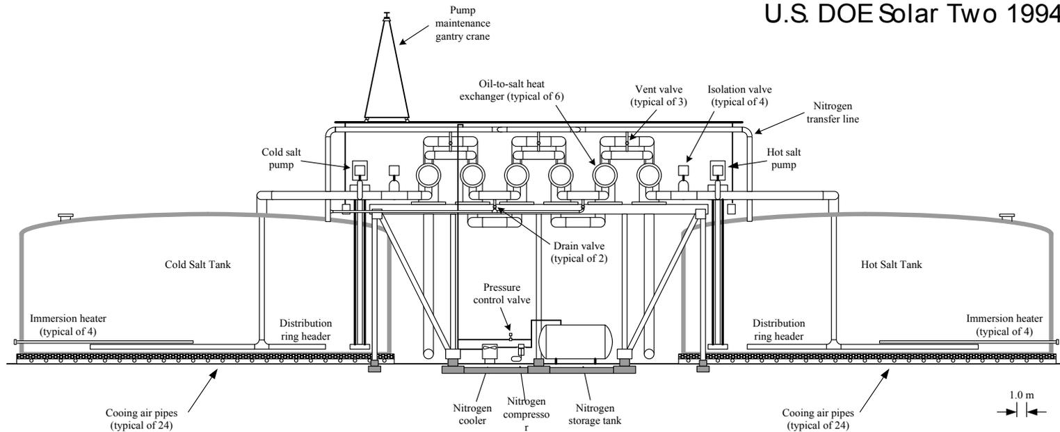
Indirect 2-tank TES configuration used for non-Abengoa parabolic trough plants in Spain
