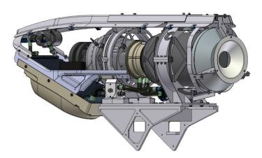
PCM volume is sized to generate 3kWh net electric power from TES; about 35 kg PCM
