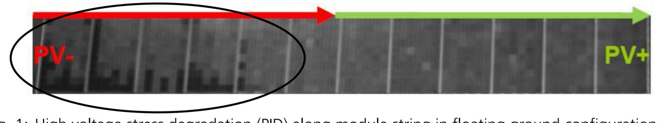
Fig. 1: High voltage stress degradation (PID) along module string in floating ground configuration [1]
