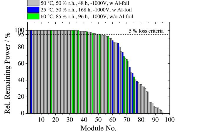
Fig. 6: Remaining power summarized for all tested modules (95 tested modules)
