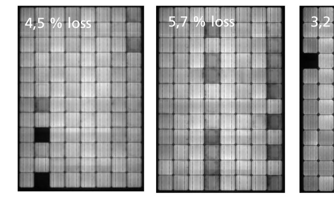
Fig. 8: Typical degradation pattern for different test approaches; left: setup 1; right: setup2
