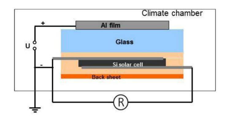
Fig. 4: Scheme of experimental setup 1
