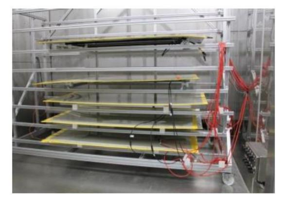
Fig. 5: Experimental setup 1 at Fraunhofer CSP with Al-foil covered PVC sheets
