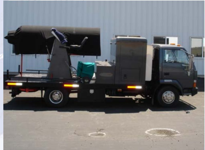
Survival wind testing by Jet Engine
