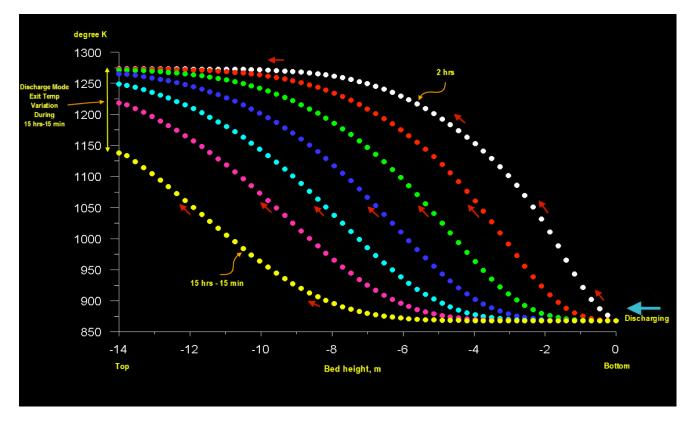
The exhaust air from the turbine enters at the right (tank bottom) and exits at the left. The exit temperature drops over time, and with it the power output of the turbine. The turbine of choice has high part-load efficiencies. In addition, depending on customer demand, fuel can be added in the combustor to maintain full power.
