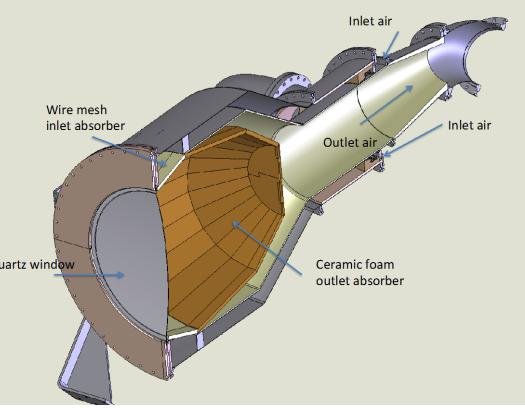
Note that the quartz window has been modified in the final design from a single piece to multiple panes
