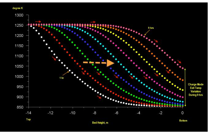
The receiver-heated air flows from left (tank top) to right (tank bottom). Variable speed flow enables near-constant inlet temperatures. In this analysis, the outlet temperature is allowed to rise to as high as 750C.
