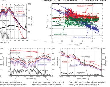
Temperature deviations of each sensor according to temperature from  $V_{ac}$ .
