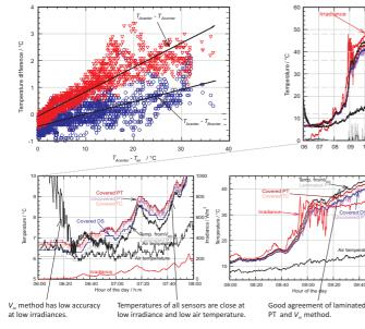
Test by shading the PV module shows adeqate time response of all sensors.
