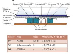
Locations of laminated PT sensors behind two cells in the middle area of the PV module and a photo of temperature sensors arrangement at the back side of PV module.
