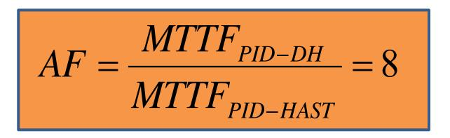
The acceleration factors (AF) here are simply computed as the ratio of the mean time to failure (MTTF) for the two tests. In the case of the PID tests, parts failed too rapidly to capture a measurement near a 5% power loss, and therefor there is significant uncertainty determining the TTF. Clearly, however, there is a significant acceleration of the dominant degradation mechanism.
