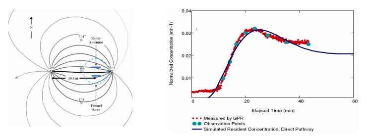
GPR measured tracer breakthrough at project field site (Becker and Tsoflias, WRR, in press)
