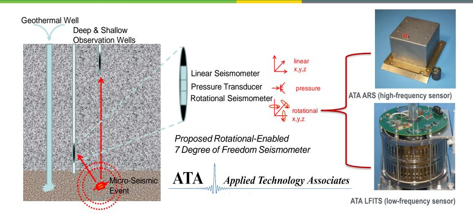
Rotation-Enabled 7-DOF Seismometer
