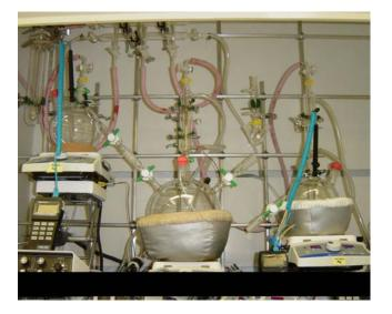
Approach 2: Photograph of high-reaction-volume synthesis set-up for up-scaled quantum dot production.
