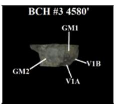
Powdered, homogenized samples weighed and analyzed for  $\delta^{13}$ C and  $\delta^{18}$ O on Gas Bench Device linked to a gas Isotope-Ratio Mass Spectrometer at WVU Stable Isotope Laboratory.
