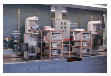
Example of flow-through system configuration
