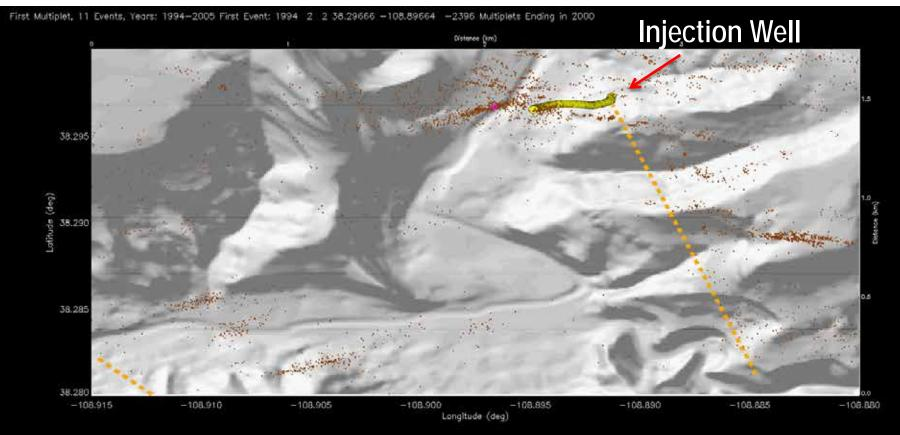
Validation of Coda Wave Interferometry: Detection of Velocity Changes near Injection Wells. Multiplet set 9 (frame 2 of 8)
