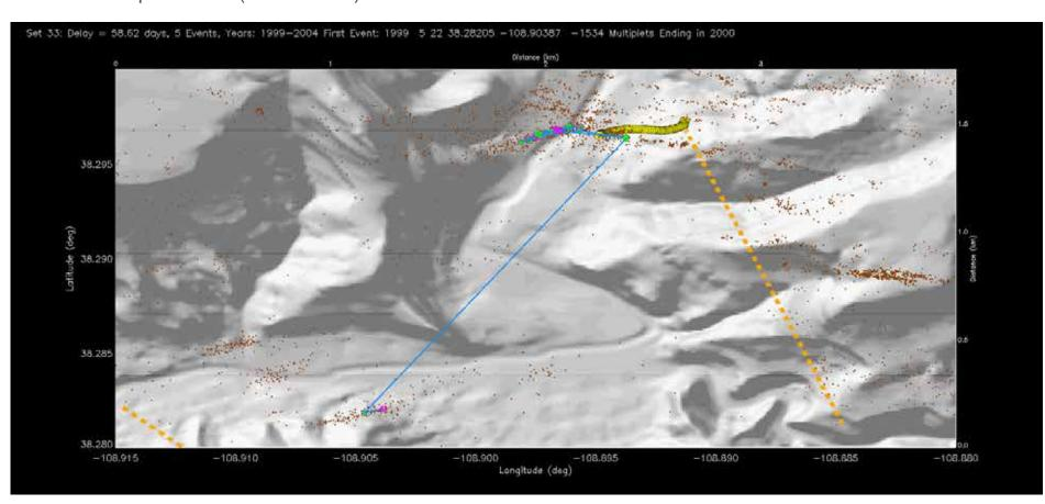
Validation of Coda Wave Interferometry: Detection of Velocity Changes near Injection Wells. Multiplet set 34 (frame 7 of 8)
