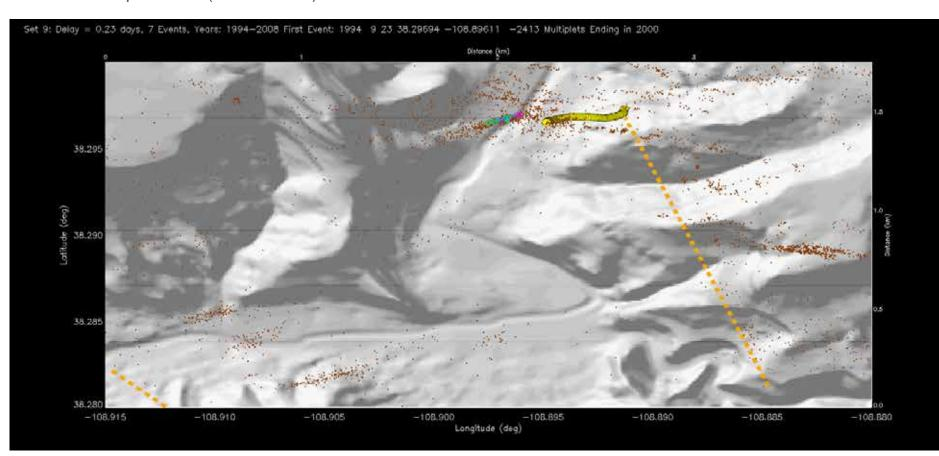
Validation of Coda Wave Interferometry: Detection of Velocity Changes near Injection Wells. Multiplet set 25 (frame 3 of 8)
