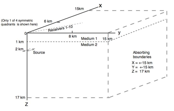
Figure 1. Problem setup for the test case LOH.1 as shown in Day (2001).
