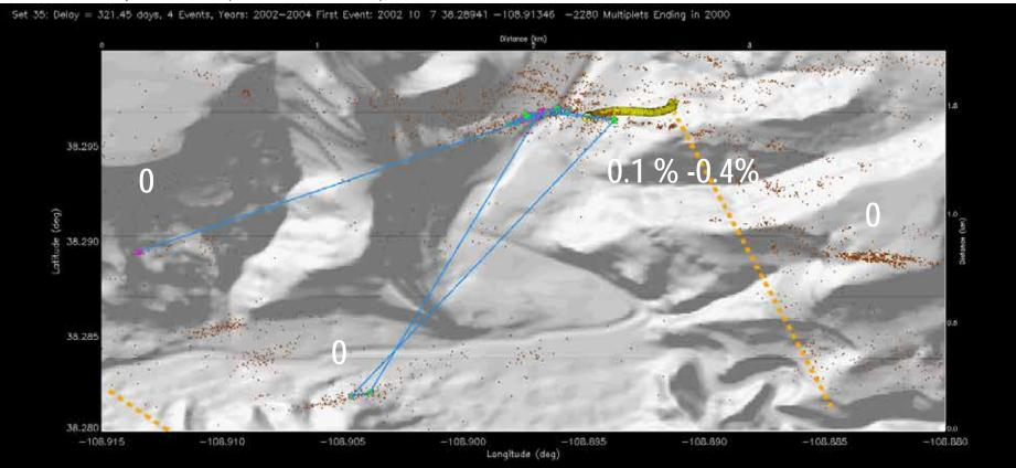
Validation of Coda Wave Interferometry: Detection of 0.1%-0.4% velocity changes within 200 m of the. Paradox Valley Injection Well. Testing also confirmed null results for multiplets located > 1 km from the well.
