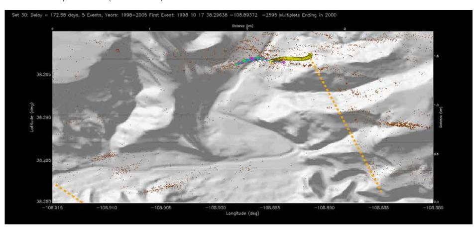
Validation of Coda Wave Interferometry: Detection of Velocity Changes near Injection Wells. Multiplet set 32 (frame 5 of 8)
