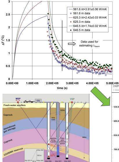
Well logs for Ktzi201 and Ktzi202 showing temperature changes (dT) during DTPS heating and calculated thermal conductivities (TC) along with well layouts and lithologies [after Förster et al., GHGT-9, 2008].
