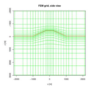
Topographic Test Model (Coarse Discretization) (after Nam et al., 2007)
