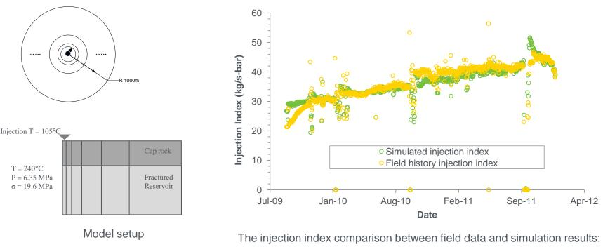
The injection index comparison between field data and simulation results: The well injection index increased with time indicates well stimulation due to cold water injection which can be captured by the simulation.
