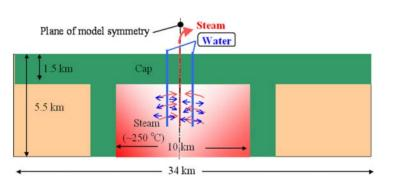
Schematic of model geometry for coupled THM modeling of steam production and water injection at the Geysers Geothermal Field
