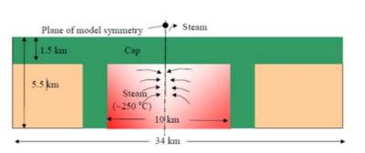
Schematic of model geometry for coupled THM modeling of steam production at the Geysers Geothermal Field
