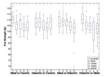
Adhesion of dielectric(5951), metal(5771) and alumina substrate shows very little degradation at 300C
