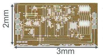
The op amp circuit consists of 15 transistors and 17 resistors
