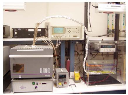
• Highly accelerated life testing (HALT) methodologies were employed with both voltage and temperature as acceleration factors to determine lifetime at 300° C
