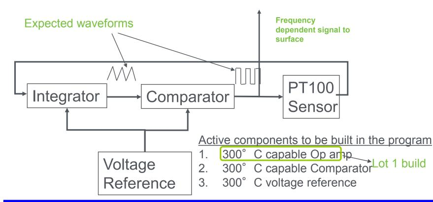
This circuit can be configured to convert different sensor signals to different frequencies so that we can transmit the signals on a single channel
