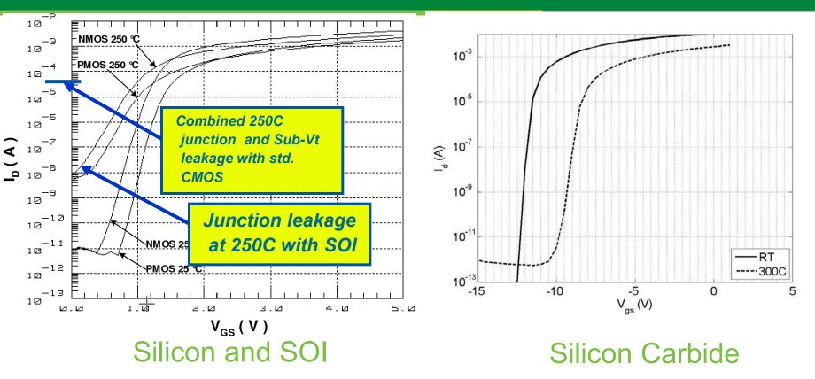
The band gap of SiC (3.26 eV) compared to the band gap of Si (1.12eV) is the reason for the low leakage of p-n junctions at high temperatures
