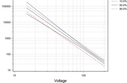
Value: 0.10uF, 50V, H dielectric Temperature: 300C Voltage Bias: 290, 200, 100 Model parameters: n=3.67 using 100 and 200V Estimated Life: 17254 hrs at 25V
