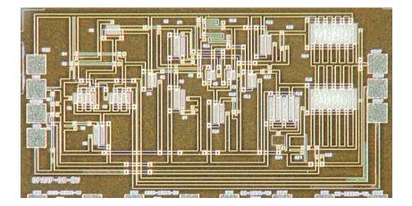
Silicon Carbide Integrated Circuit
