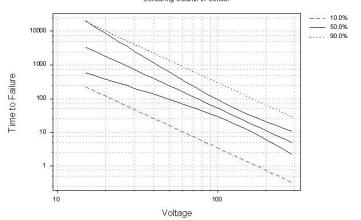
Projected lifetime of TRS capacitor at 15V is excess of 1000 hours at 350C
