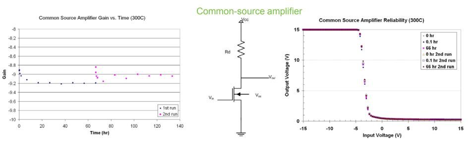
• The circuits were stressed so that maximum current flows through the transistor at 300°C
