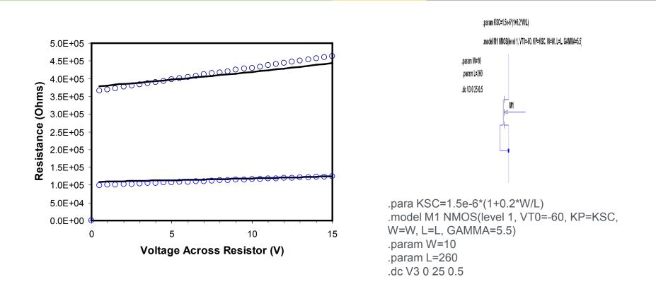
Resistors are modeled as a transistor with gate and source shorted Resistor behavior depends on geometry and need standard
