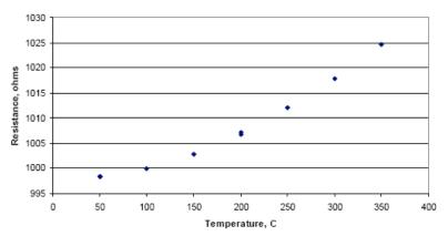
1 k $\Omega$  thick film resistor
