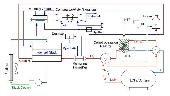
Figure 1 Automotive fuel cell system with organic liquid carrier hydrogen
