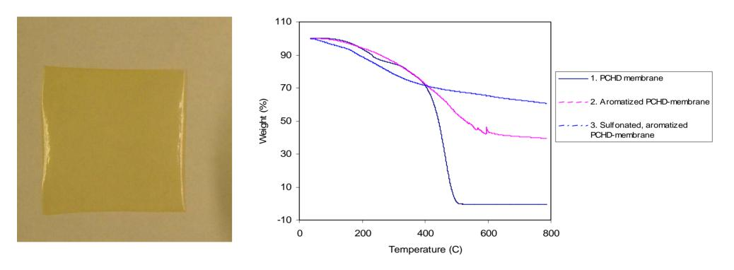
Left: A photograph of a cross-linked 2.5"X2.5" PCHD membrane; Right: TGA curves 1) for the cross-linked PCHD membrane, 2) after aromatization, 3) after aromatization and sulfonation
