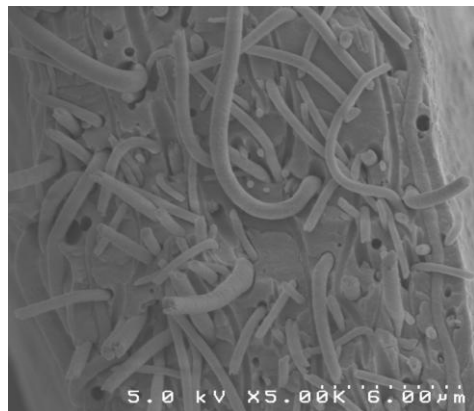
Nafion® matrix (~70 vol%), polyphenylsulfone nanofibers
