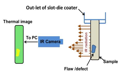
Schematic of IR thermography method to detect flaws in dry electrodes
