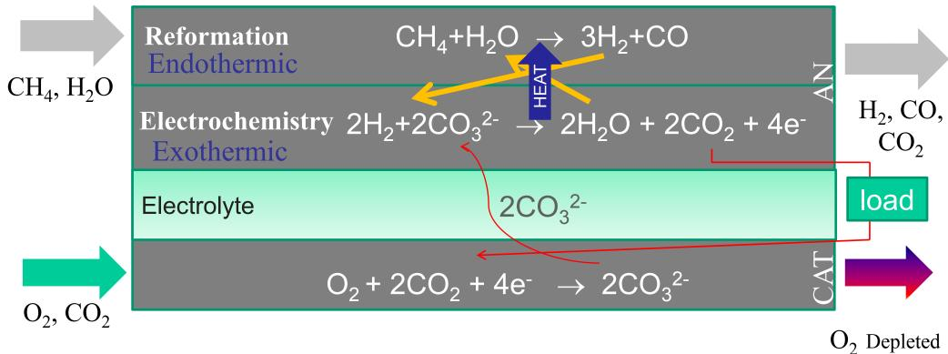
Air Flow and parasitic blower power can be reduced
