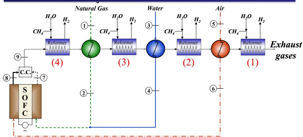
Placement of a reformer in different locations: Configuration 1 ⇒ reformer after the air preheater, Configuration 2 ⇒ reformer after the water preheater, Configuration 3 ⇒ reformer after the natural gas preheater, Configuration 4 ⇒ reformer after the combustion chamber.
