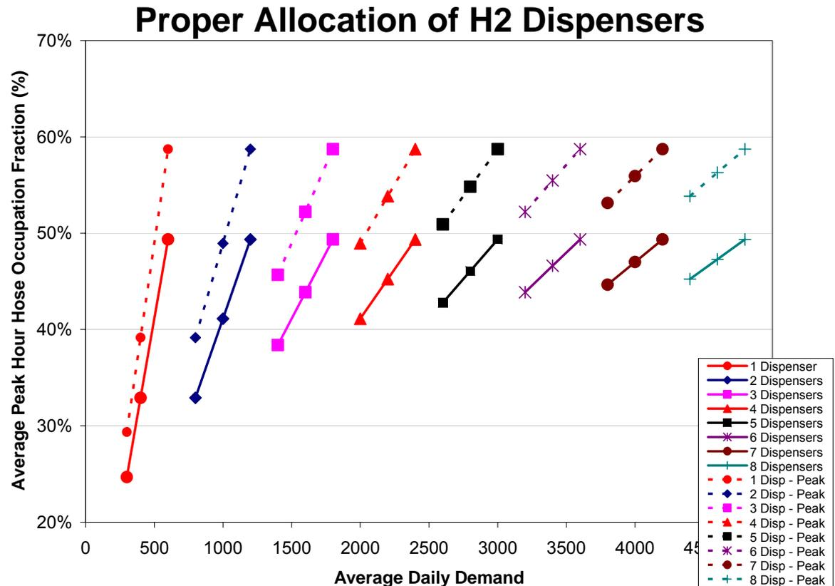
**Assumes: 6 kg<sub>H2</sub> vehicle tanks, 75% average fill, 3 min. linger time, 1.67 kg/min hose flow rate**
