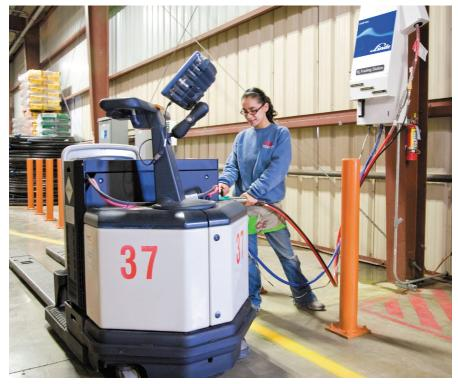
Operator makes hydrogen dispenser connections to a Class 3 material handling vehicle.
