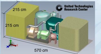
Conceptual layout of a net 400 kW SOFC power system
