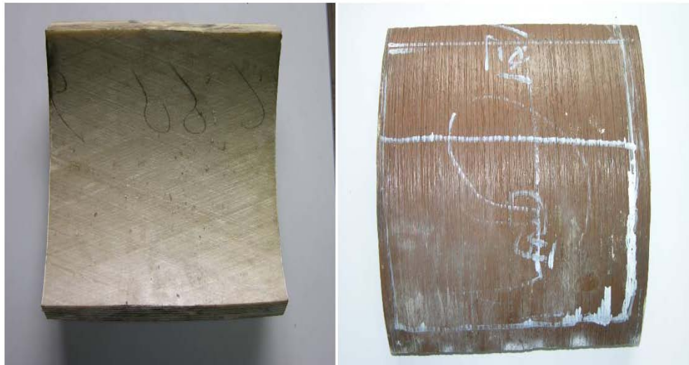
Figure 8 Internal and External Surfaces of Cylinder Liner
